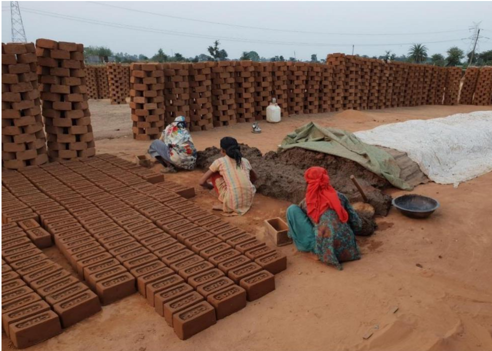
Figure 2. Mudiya Kheda, near Chhola in Madhya Pradesh. Commercial adobe manufacture undertaken in a rural context seasonally. (Source: CarstenHermann)
